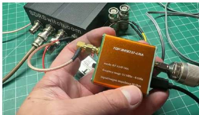
Figure 5 — A TQP3M9037-LNA amplifies the signal before it reaches the SDR.
