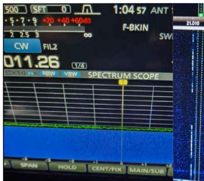
Figure 2 — An IC-7610 and an Airspy HF+ SDR running side by side on SDR Console .
