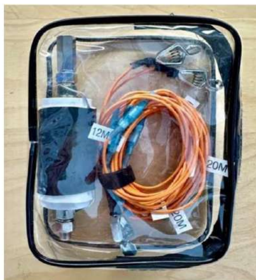
Figure 7 — The packaged radials and 40-meter coil.
