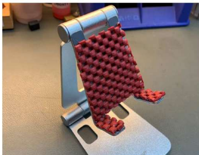
Figure 4 — Glue small pieces of drawer liner material to the stand to provide additional support. [Dino Papas, KLØS, photo]
