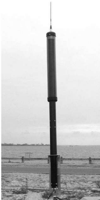
Figure 1 — From The ARRL Handbook , Figure 21.72: The screwdriver-style remotely-controlled whip antenna. A small motor in the base mast moves a coil past contacts at the top of the metal base section. The top whip section is attached to the top of the coil. As the coil moves out of the mast, more inductance is connected in a series between the base section and top section. Screwdriver antennas are popular because they offer multiband coverage. [Joel Hallas, W1ZR, photo]
