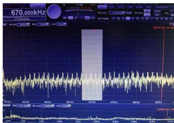
Figure 6 — The interfering signal was strongest at around 670 kHz. It appeared on my SDR receiver display as a row of jagged peaks. It was quite noticeable on HF as well. [Kraig Krist, KG4LAC, photo]
