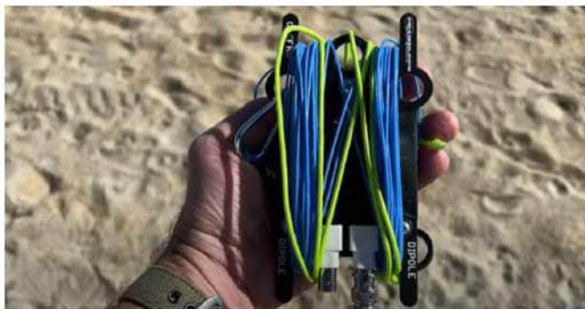
Salty Walt, K4OGO, shows the small size and compactness of one of his favorite portable antennas.
