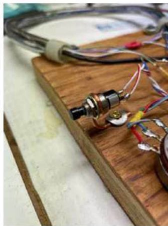
Figure 5 — In this close-up view, you can see how a pushbutton is held in place with a loop of copper wire that is secured to the wood plank with a screw. [Jim Kocsis, WA9PYH, photo]
