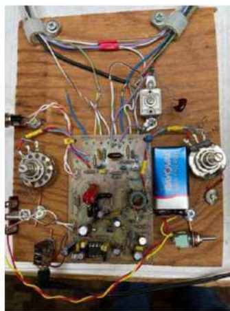
Figure 6 — By using this technique, all of the interface components are firmly held in place for testing. Assuming the testing goes well, they can be easily removed for permanent installation in a suitable enclosure. [Jim Kocsis, WA9PYH, photo]
