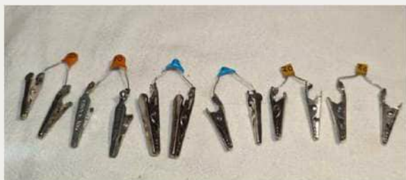
The author's capacitor compensation kit.
