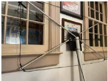
Figure 9 — DXE flag antenna noise loop as built.
