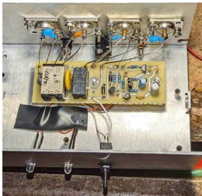
Figure 3 — QSK switch internal view.
