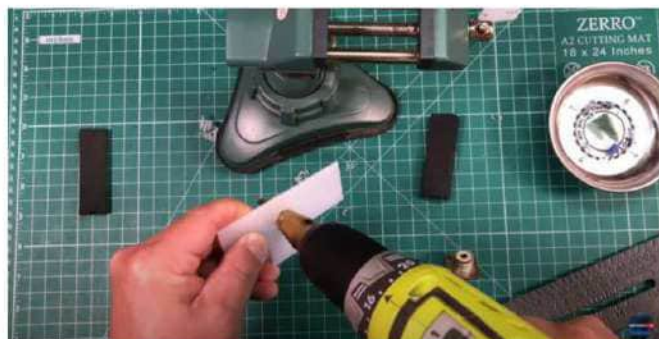
Mike, K8MRD, demonstrates how to build your own antenna insulator.
