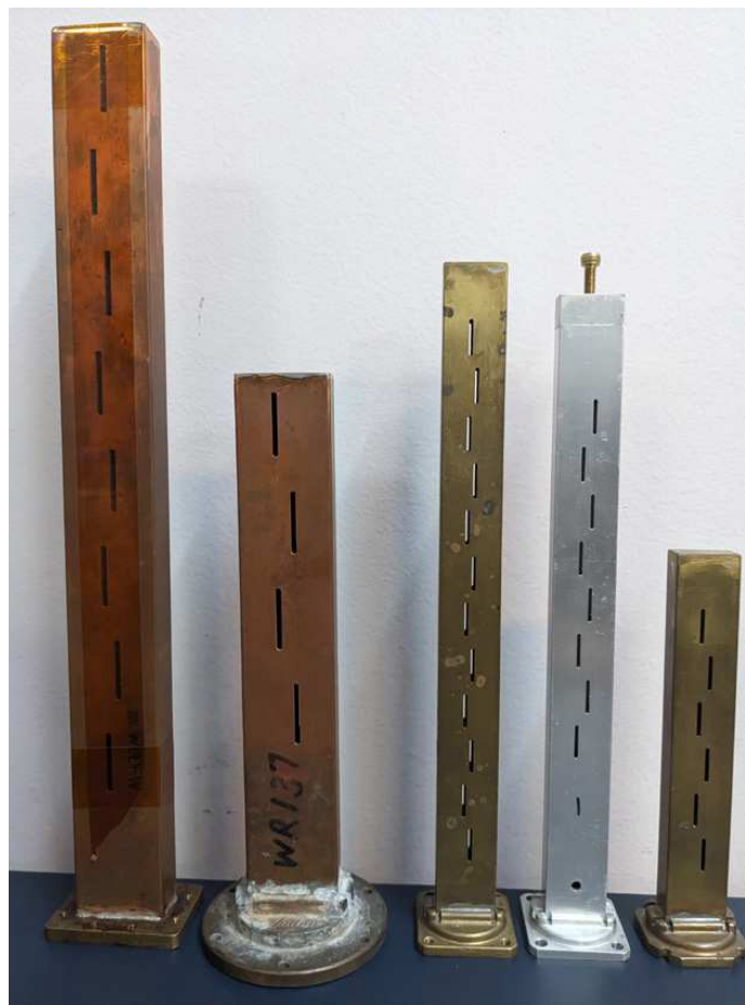
Figure 1 — Various waveguide slot antennas from left to right: WR-137 antennas with 16 and eight slots for 5760 MHz. WR-90 antennas with 24, 16, and 12 slots for 10368 MHz. [Glenn Robb, KS4VA, photo]
