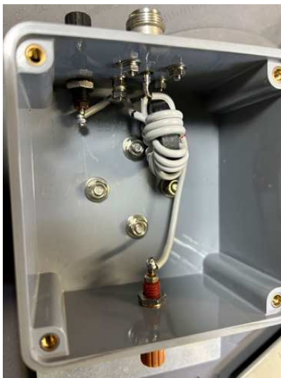
Figure 4 — A 450 to 50 \Omega balun.
