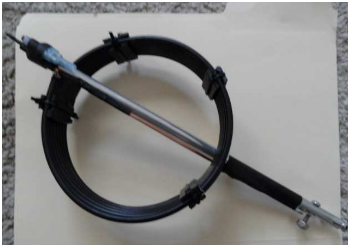
Figure 3 — The trap, which is resonant near 80 meters. The aluminum tube has no effect on the trap.
