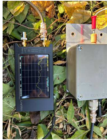
Figure 5 — Measuring at ground level into the vertical feed wire using a LiteVNA-64. Four short radials were used as a counterpoise.
