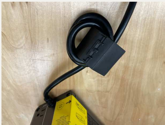
Figure C — Snap-on choke used for the APC unit.
