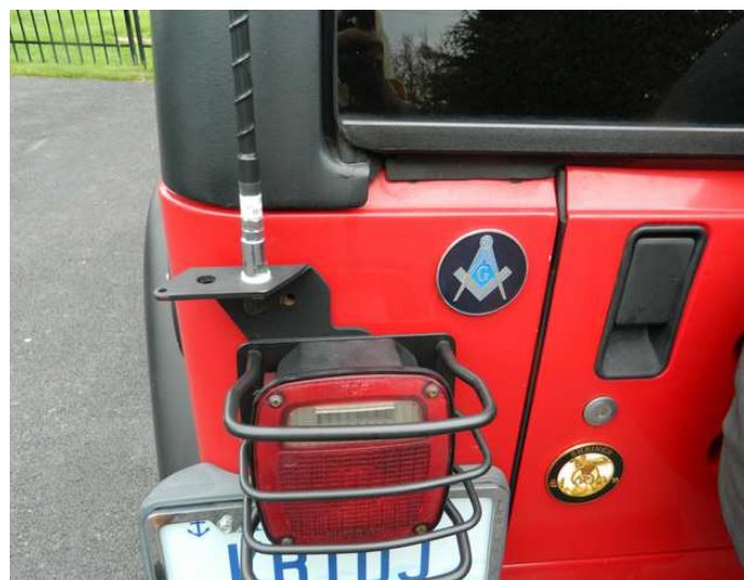
Figure 4 — The rear driver's-side 5/8-24 antenna mount.
