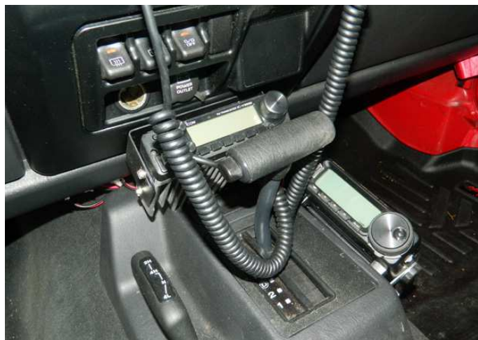
Figure 1 — Installing radios as close to the vehicle's floor as possible can help keep equipment out of sight.
