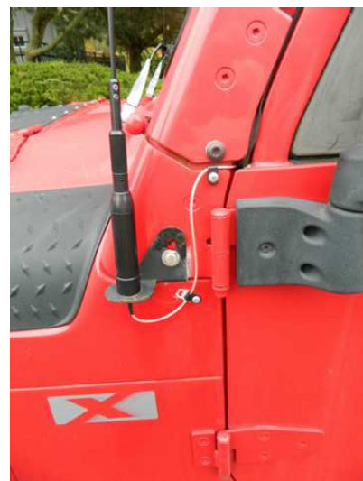
Figure 2 — The Comet SBB-25 installed on the driver's-side cowl.
