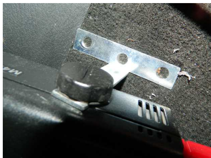
Figure 5 — One of the steel brackets used to mount the FT-891 to the side of the center console.
