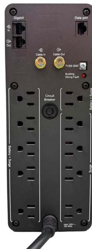
Figure 2 — The APC Pro BN1500M2 rear panel.
