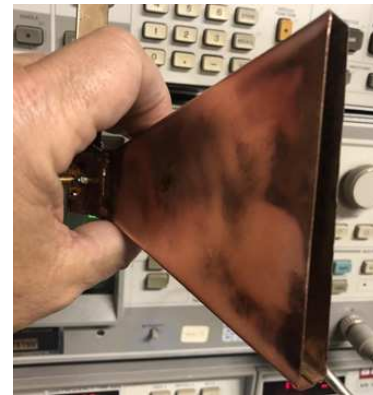
Figure 4 — A sectoral horn for 10368 MHz made of copper by John Swiniarski, K1OR. [John Swiniarski, K1OR, photo]
