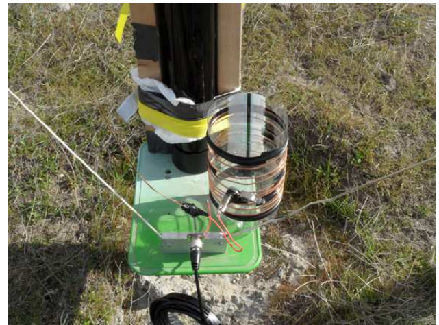
Figure 4 — The hairpin coil, feed point, and start of the radials. Note that the coil form can also serve as a rain gauge unless drain holes are used.
