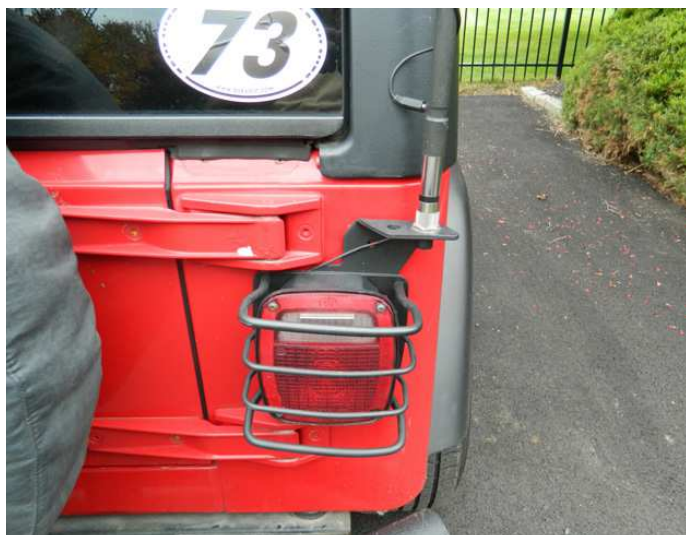
Figure 3 — The rear passenger's-side antenna mount, with the SO-239 connector.
