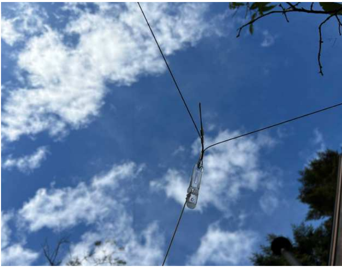
Figure 2 — Corner supports of the wires.
