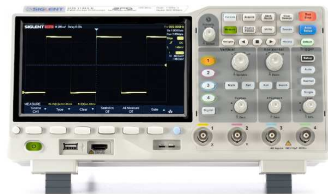
Figure 7 — The Siglent Technologies SDS1104X-E. The LAN and USB connectors on the lower left are used to input programs, control the unit, update the firmware, and save screen data.
