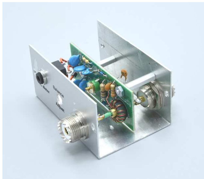
Figure 12 — Inside the SWR/power sensor.
