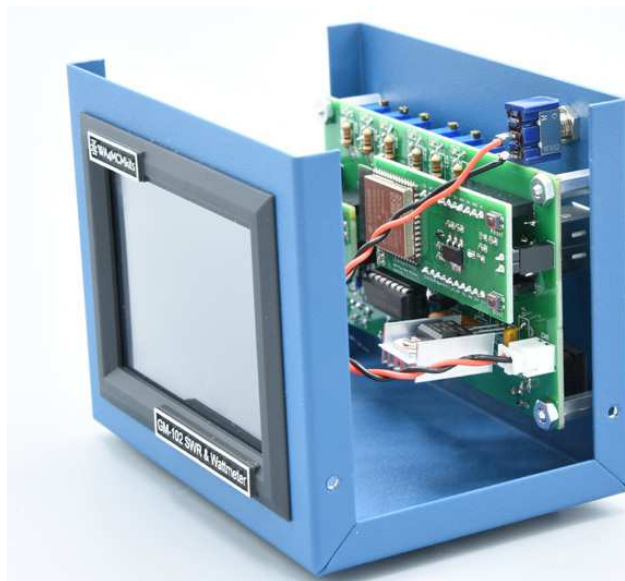
Figure 11 — The main unit assembled and ready for calibration using the blue variable resistors along the top left edge of the PCB.
