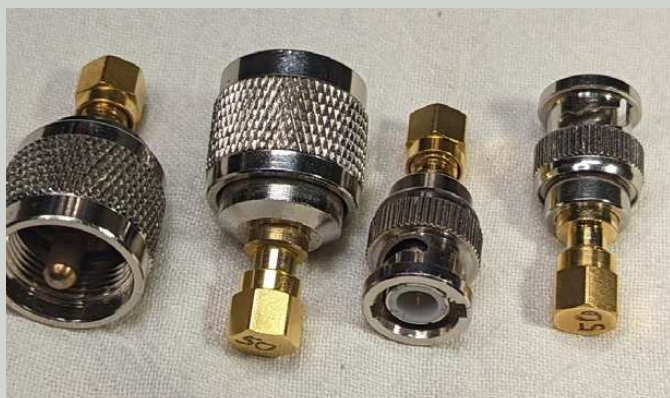
Figure 5 — UHF and BNC 50 \Omega terminations.
