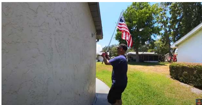
Bob, KD4BMG, setting up the wall-mounted flag that will serve as a stealth antenna in plain sight.
