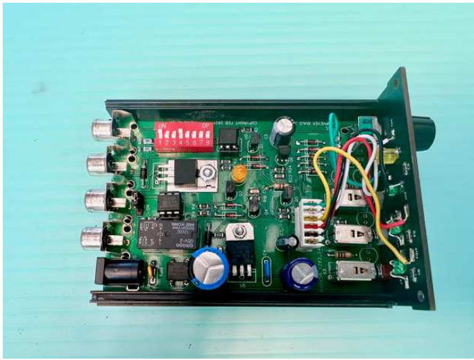
Figure 3 — Inside the ampkeyer. The solid-state relay was not installed on this PCB. Many of the resistors are SMD. The steering diodes are in the upper right, while the power supply components are in the lower left of the PCB. PCB material is used for the front and rear panels. Small LEDs are pressed into the PCB.
