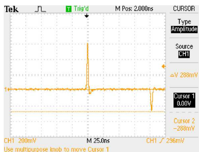
Figure 9 — Reflected pulse/cable-loss measurement.
