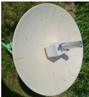
Figure 1 — Measuring NF using a small horn to compare sun, sky, and ground noise. The reflector reduces unwanted ground noise when measuring sun and sky noise.
