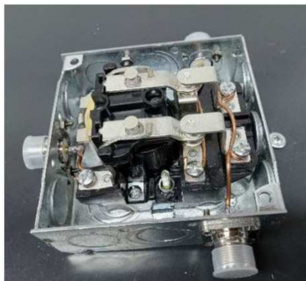
Figure 3 — Mounting of the relay and the SPDT wiring. [Robert J. Zavrel, W7SX, photo]
