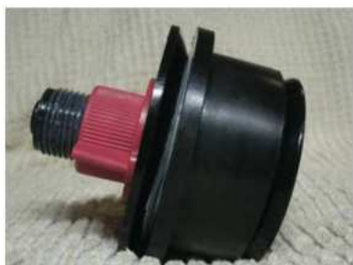
Figure 5 — A test plug is used to temporarily seal a pipe for testing under pressure. [John Dewey, KA9CAR, photo]
