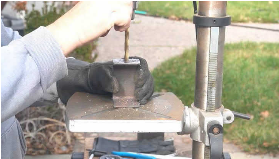
Chuck, KK6USY, demonstrates drilling into the C channel while building his clamp.
