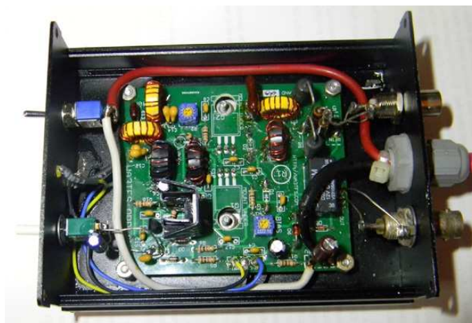
Figure 1 — An interior view of the linear amplifier.
