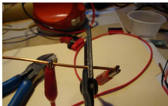
Figure 3 — In this image, both ends of a clip lead are pressed into service. When I cut between the clips, both pieces of wire will remain nearby. [Phil Karras, KE3FL, photo]
