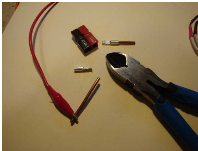
Figure 2 — Once this wire is secured within the Powerpole tab, the clip lead will keep the excess wire from flying away when cut. [Phil Karras, KE3FL, photo]
