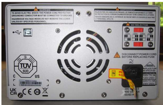
Figure 10 — Two three-position slide switches allow selection of line voltages 100, 110, 220, and 230 V at 50/60 Hz.
