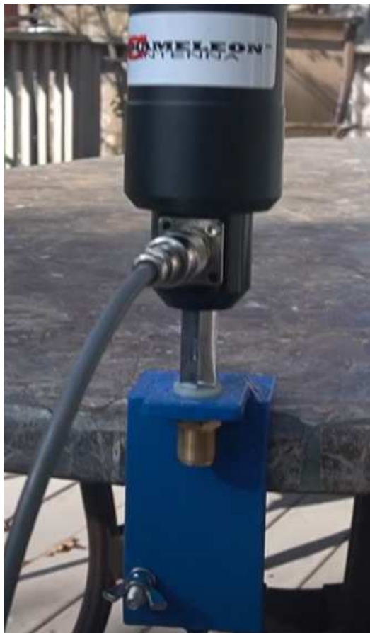
Chuck, KK6USY, demonstrates the completed C-clamp antenna mount.
