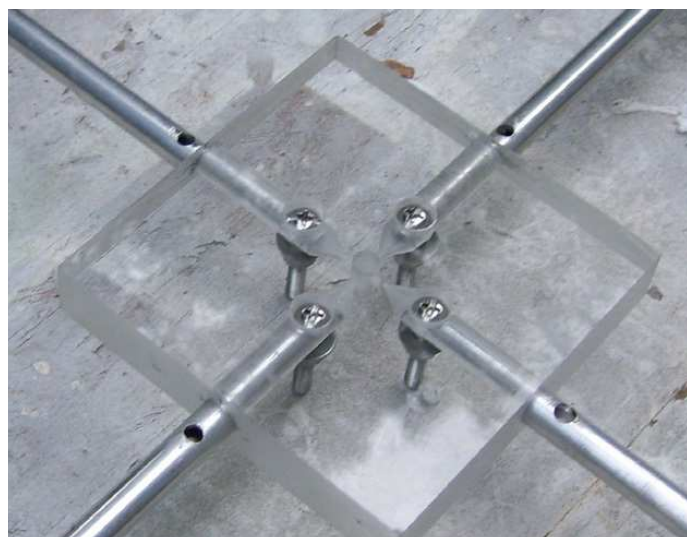
Figure 2 — The center support, consisting of a 4 x 4 x \frac{3}{4} -inch-thick block of clear acrylic plastic.
