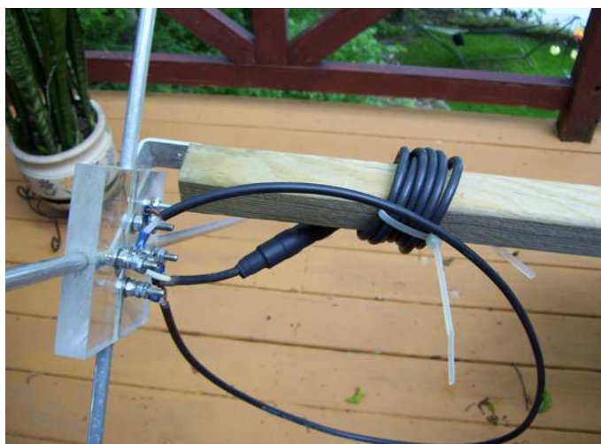
Figure 3 — The fully assembled center support, which includes the delay line.
