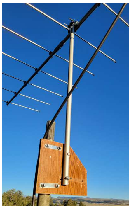
Figure 1 — The homebrew antenna polarity-switching mount. The Yagi is shown in its horizontally polarized position. [Stephen Peterson, KI7L, photo]
