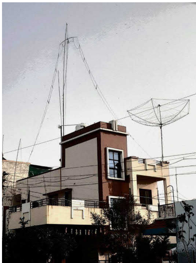
Figure 1 — Kishh Galnimbkar's, VU2MZT, antennas. A fan dipole for 40 and 20 meters is on the left, and a hexbeam is on the right. [Kishh Galnimbkar, VU2MZT, photo]
