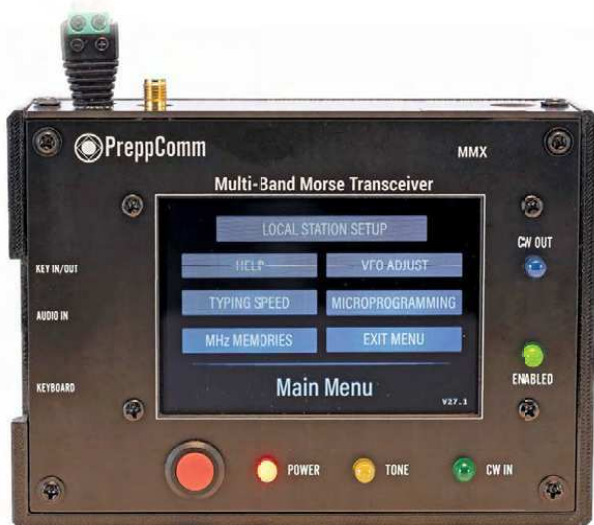
Figure 2 — The PreppComm MMX main menu has six choices, including the internal HELP system.
