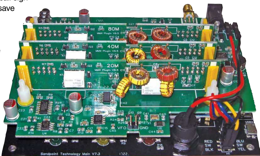
Figure 1 — Internal view of the PreppComm MMX, showing the three band modules (80, 40, and 20 meters).
