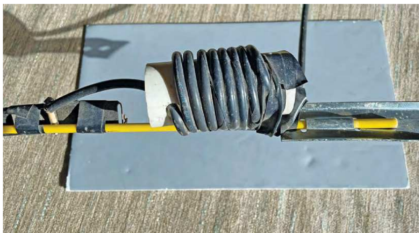
Figure 1 — An “ugly balun” for a J-pole made by wrapping several turns of coax around a short length of plastic pipe. On 2 meters, this provides enough inductance to keep common-mode current from coming down the coax. This coax coil does not affect what is inside the coax except to add length to the transmission line. This simple coax coil is called a balun because the J-pole is a balanced antenna, and the coax is unbalanced. The coil keeps the balanced antenna currents separated from the coax’s outer shield, thus connecting the balanced antenna to an unbalanced feed line.
