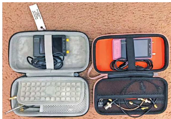
Figure 1 — Two open cases with test instruments. Note the straps to hold the instruments in place and the pockets for cables and other components. [Bruce MacAlister, W4BRU, photo]
