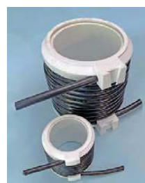
Figure 2 — Completed small 40-meter and large 80-meter un-ugly baluns.
