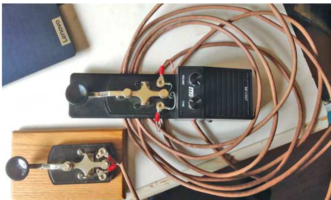
Figure 4 — The finished shared oscillator system. The oscillator sounds whenever either key is closed. [Jakin Messer, AG7WW, photo]
