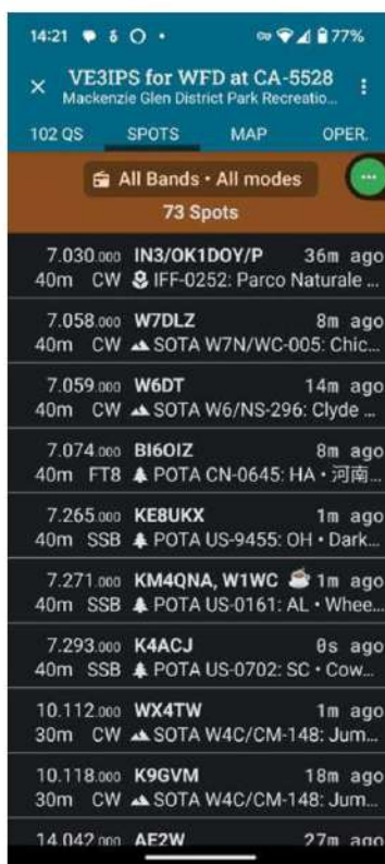
Figure 4 —The PoLo "Spots" tab. Clicking a spot populates the QSO tab with all contact details, enabling quick responses.
