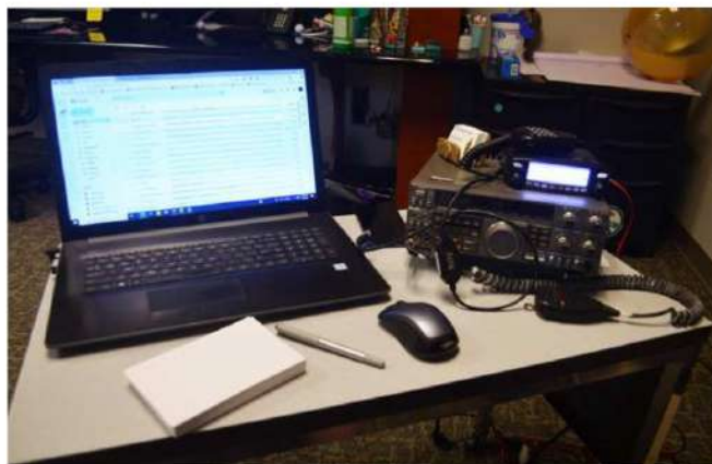
The WBTW News station amateur radio setup, which includes a laptop to monitor the weather, a Kenwood TS-440S HF transceiver, and a Yaesu FTM-100D for VHF communications. The stack of index cards is used to pass messages to the producer. [Gordon Mooneyhan, W4EGM, photo]
