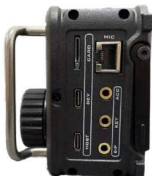
Figure 2 — The Xiegu X6200 right side, showing the mic, data, key, and audio interfaces.
