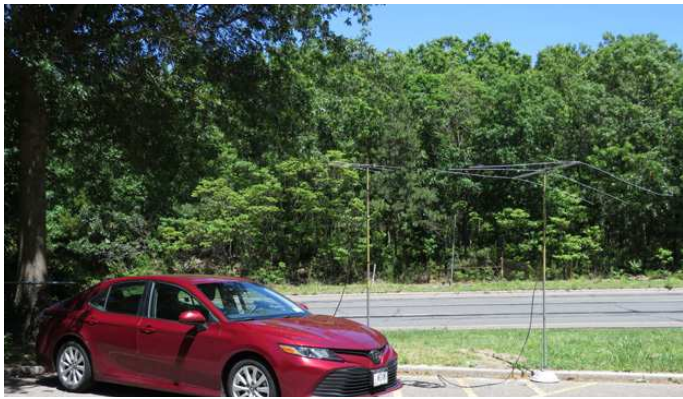
Figure 2 — The author's low-power 2- and 6-meter setup for the 2025 ARRL June VHF Contest. For this event, he operated on a hilltop and used three-element beams mounted on umbrella stands, and he set the masts at 10 feet high.
