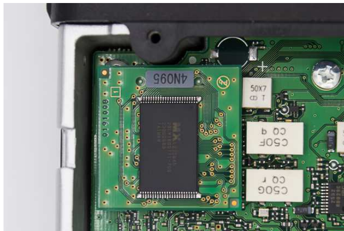
Figure 4 — The optional FVS-2 Voice Guide Unit after installation in the FTM-150RASP.
