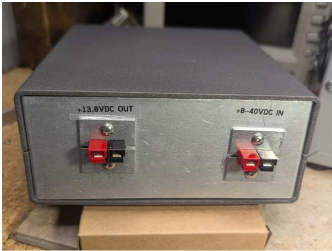
Figure 11 — The dc Powerpole interfaces.
