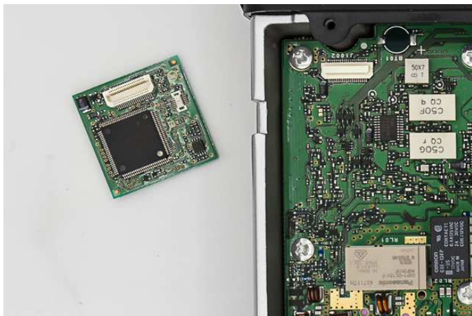
Figure 3 — The optional FVS-2 Voice Guide Unit before installation in the FTM-150RASP.
