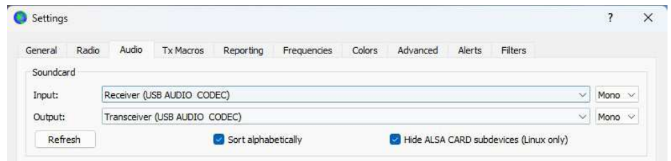
Figure 3 — Setting the input and output device on WSJT-X.
