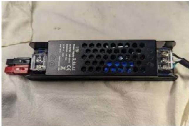
Figure 1 — The 12 V 5 A power supply.
