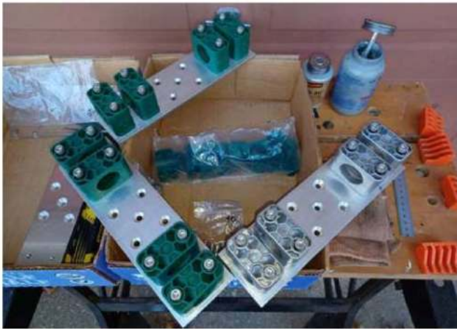
Figure 3 — The elements are mounted on an aluminum plate using a STAUFF-style tubing clamp and stainless-steel hardware.
