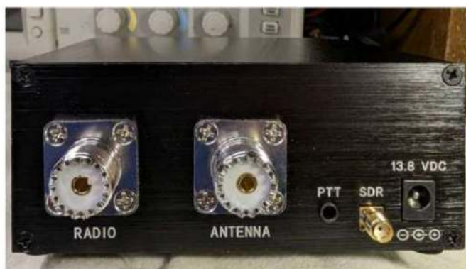
Figure 9 — Rear of the SDR TX/RX switch.
