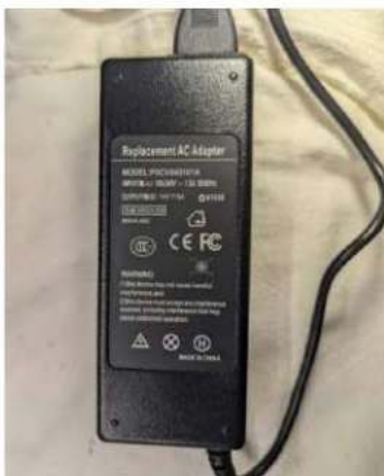
Figure 2 — The 14 V 6 A power supply.
