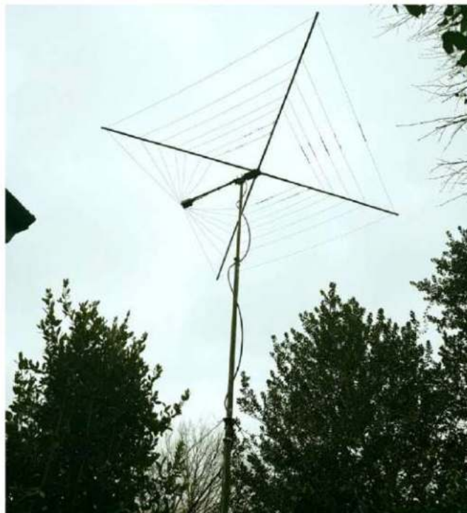
Figure 2 — David Webber's, GØPBS, cobweb antenna. A cobweb antenna is a fan dipole that is wrapped on itself. It is a compromise antenna. One compromise is that for any given band, it doesn't cover the entire band and must be tuned to cover the part of the band that is desired. Another compromise is that the gain is 2 or 3 dB less than an equivalent dipole. Because the antenna is built upon the idea of a dipole, it is a balanced antenna, and radials are not required. [David Webber, GØPBS, photo]
