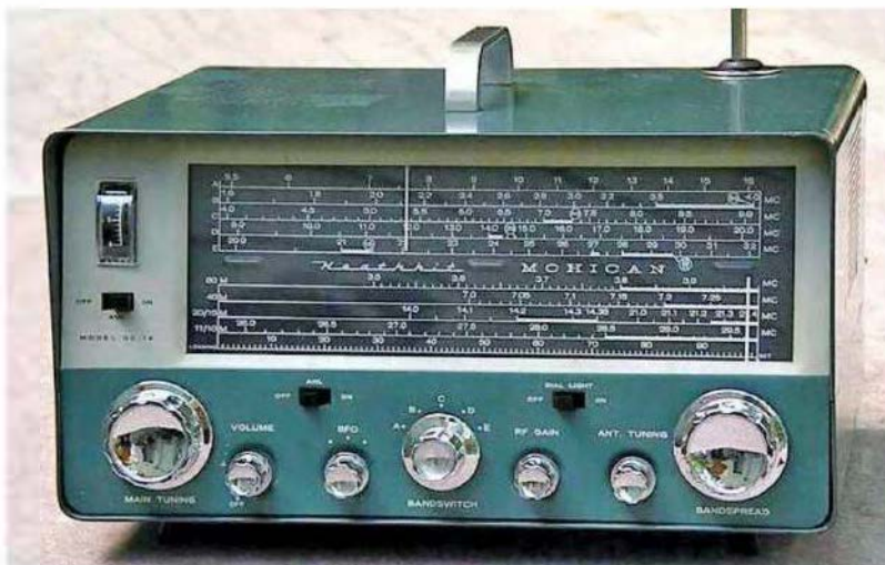
The Heathkit GC-1A Mohican receiver was the first solid-state SWL and ham radio receiver that was fully transistorized. [Photo courtesy of www.radiopics.com ]
