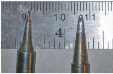
Figure 10 — The smaller tip was easier to use than the larger, standard tip in several places. The top scale numbers are centimeters; the smaller divisions are millimeters.
