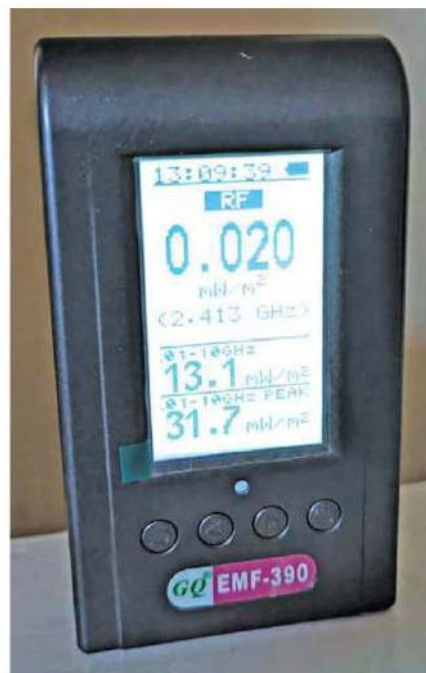
Figure 6 — The GQ EMF-390 showing Wi-Fi channel 1.
