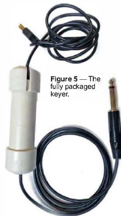
Figure 4 — The keyer installed in a PVC tube.
