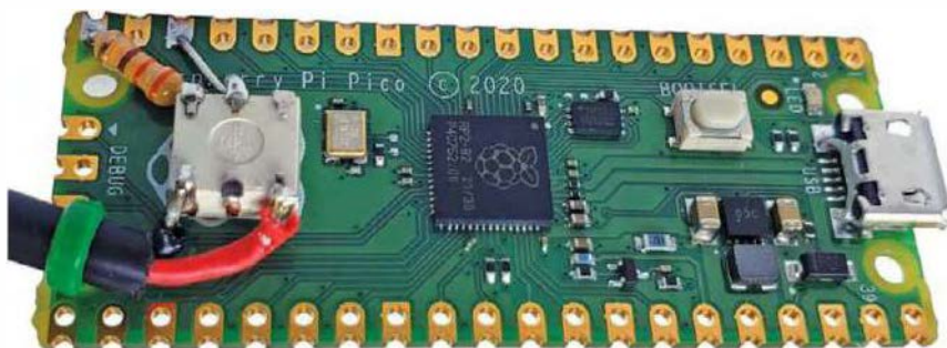
Figure 2 — The simplest version of the keyer.
