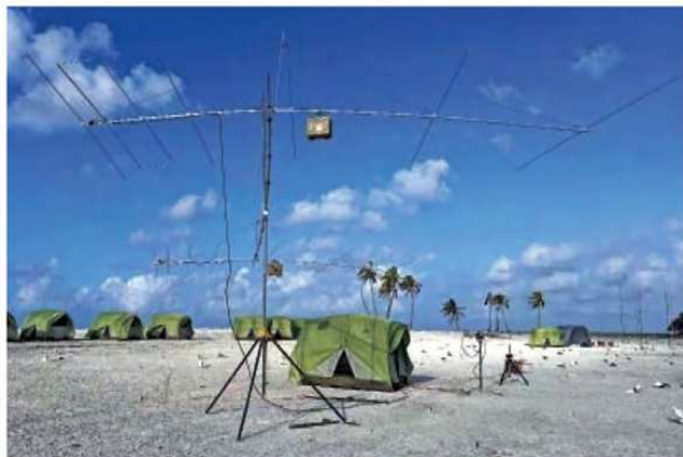
The seven-element over seven-element array that the TX5S team used for 6-meter Earth-moon-Earth (EME). Note the counterbalances. [Andreas Junge, N6NU, photo]
