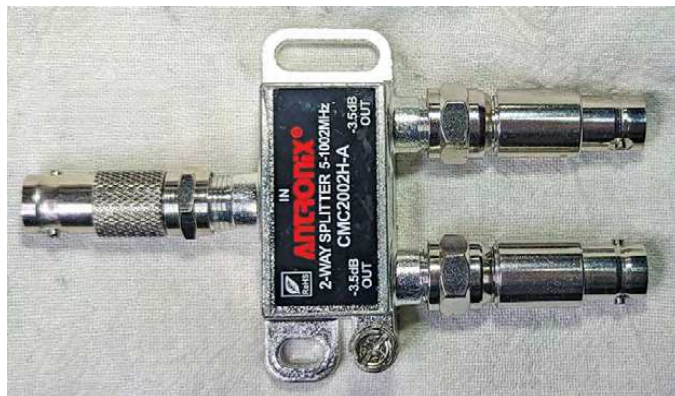
Figure 14 — The Antronix two-way 75 \Omega splitter with BNC/F adapters.
