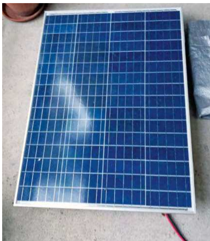
The 12 V 100 W solar panel.
