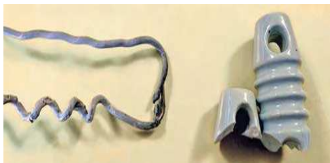
Figure 3 — One of Alex's, WB3ATF, broken ceramic insulators. An arc formed from the end of the antenna, where the voltage is the highest, to the other end, supported by a rope. The antenna wire shows signs of arcing.
