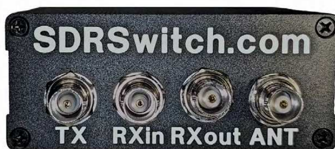
Figure 8 — The RF interconnect side of the RX-In RX-Out SDR Switch.
