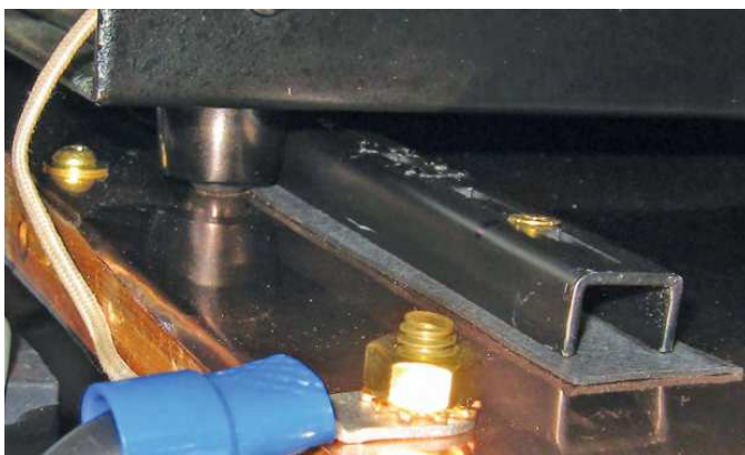
Figure 4 — In this image, pilaster strips are mounted in front of and behind the rear feet of an external speaker to prevent movement when plugging/unplugging the headphone jack. [Mark Kupferschmid, AC9PR, photo]
