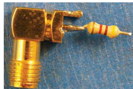
Figure 3 — A simple RF probe useful for probing and troubleshooting RF circuits, especially printed circuit boards.
