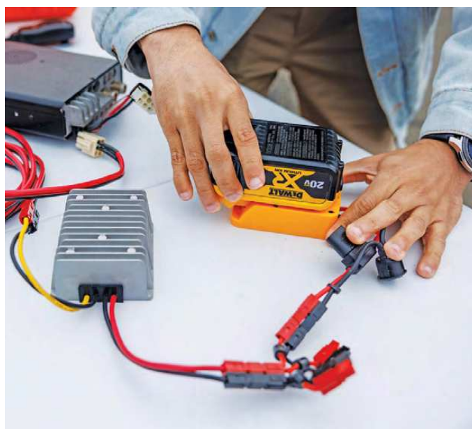
Figure 1 — When setting up for emergency communications, it can be helpful to have battery connectors of multiple brands to maximize your backup power options. A combiner for multiple batteries with Schottky diodes can also be used. [Chris Zajac, photo]
