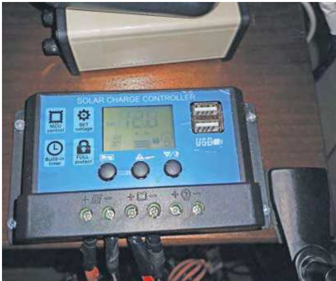
The charge controller reflecting the solar panel charges the battery and runs the radio equipment. In this photo, the solar charge controller shows the battery has been charged to 12.8 V.
