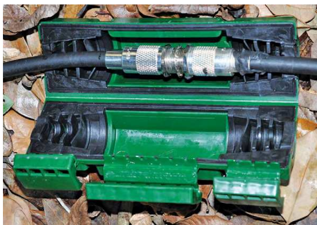
Figure 6 — A Cord Protect shield is being used to protect a feed-line splice consisting of two PL-259 connectors and an SO-239 bulkhead. [W. Derek Meche, WM5TS, photo]
