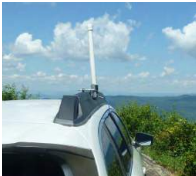
Figure 2 — Doug Allen, K4LY, operates 10 GHz portable using a waveguide slot antenna on his vehicle for quick contacts. The slot antenna is inside a PVC pipe for weatherization. [Doug Allen, K4LY, photo]
