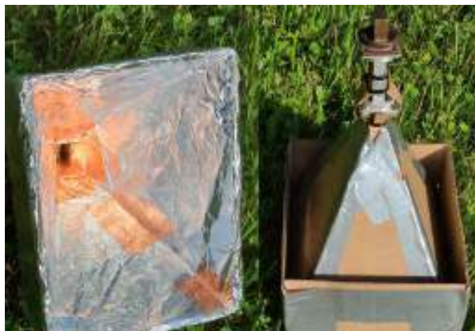
Figure 3 — A 10 GHz small WR-90 horn antenna with cardboard extender for more gain. The inside, lined with aluminum foil and copper tape, is on the left; the outside, showing duct tape and zip-tie construction, is on the right. [Paul Wade, W1GHZ, photo]
