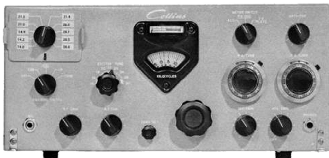
The Collins KWM-1 transceiver used a PTO that covered only 100 kHz. [Photo courtesy of www.rigpix.com ]
