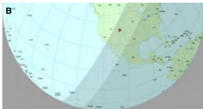
Figure 1 — Maps of Earth from DX Atlas ( https://dxatlas.com ). The first map (A) is a Mercator projection showing daylight, nighttime, and twilight. The map is distorted, particularly as you move toward the poles. On this map, twilight is depicted as a gray band, known as the “grayline.” The second map (B) shows a spherical Earth as seen from space. Note that you can set DX Atlas to display civil twilight alone, both civil and nautical twilight, or civil, nautical, and astronomical twilight.
