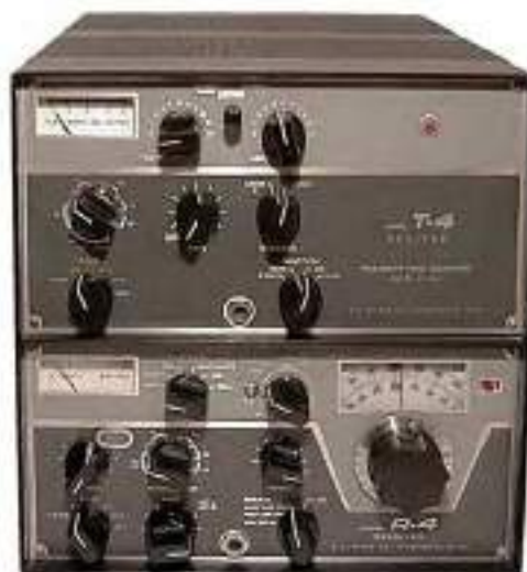
R. L. Drake's T-4 transmitter transceived only with their R-4. [Photo courtesy of www.rigpix.com ]
