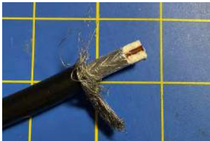
Figure 2 — Cutaway view of a Times Microwave LMR-400 coaxial cable. [Dave Casler, KE0OG, photo]
