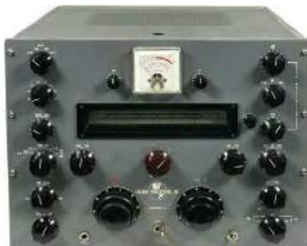
Cosmos Industries adopted Collins Radio's idea of an unswitched tunable oscillator with their Cosmophone 35 transceiver. [Photo courtesy of www.rigpix.com ]
