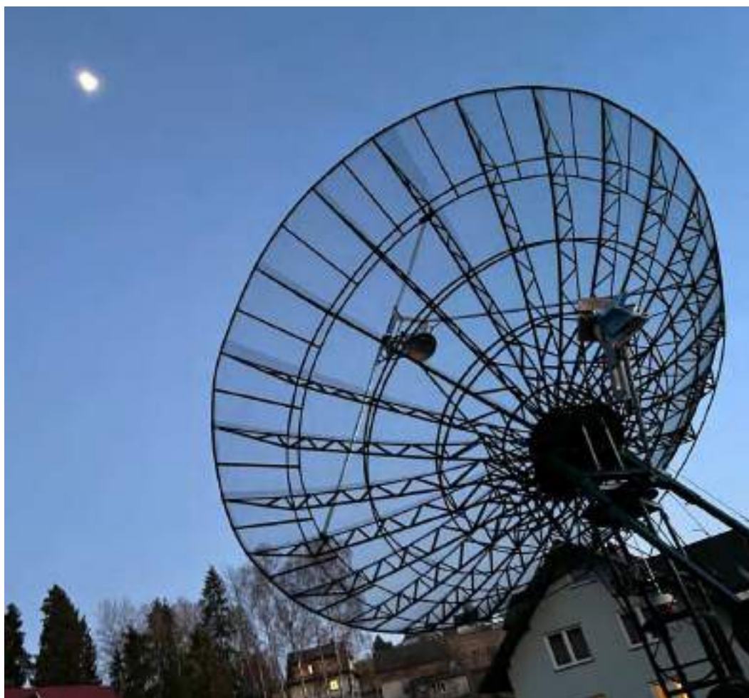
Figure 1 — Rafael's, SP9VFD, assembled 6.4-meter paraboloid dish antenna, ready to bounce signals off the moon.
