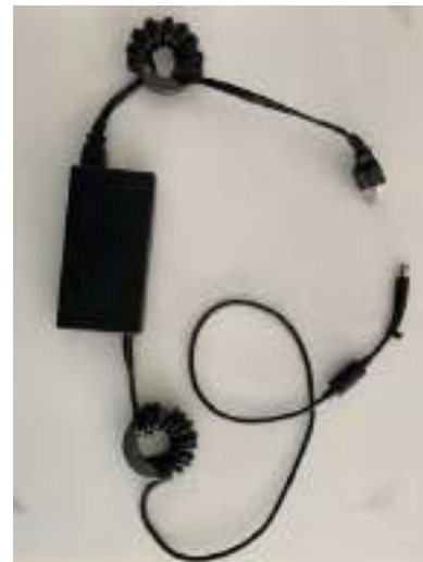
Figure 2 — The power supply brick with input and output cables wrapped around ferrite cores. [Scott Freeberg, WA9WFA, photo]
