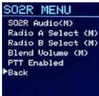
Figure 1 — The TFT display. Shown here is the SO2R menu, one of many you can select from the front panel.
