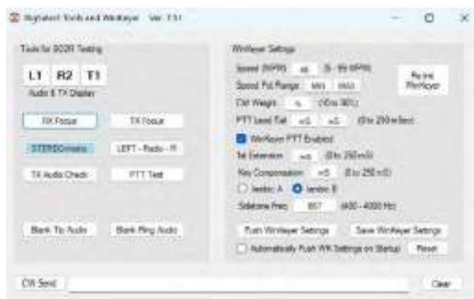
Figure 8 — The Tools and WinKeyer window can be used to set up the WinKeyer if your logging software does not provide that functionality. The tools permit testing your SO2R setup.
