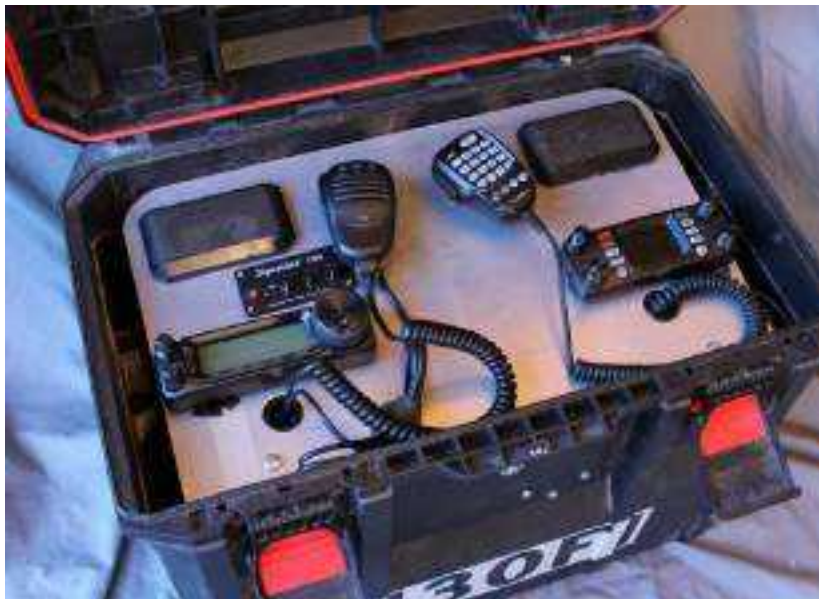
The radio go-box with the aluminum plate in the flat position.
