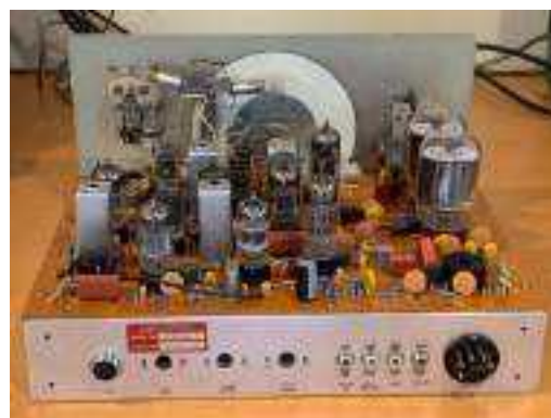
The HW-12 PCB and cleaned-up chassis.
