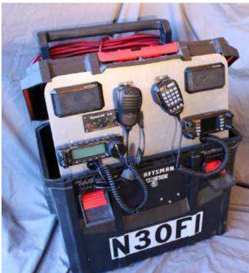
The radio go-box with the aluminum plate in the inverted position.
