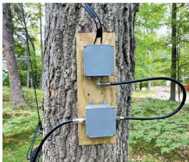
Figure 5 — The balun, toroidal transformer, and coaxial/ferrite common-mode current choke were placed in two 4 × 4-inch waterproof plastic electrical boxes and mounted to a tree.
