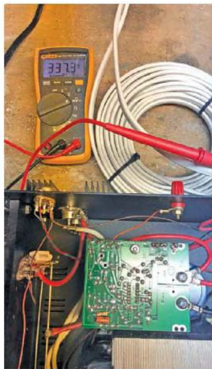
Figure 5 — I connected my digital multimeter to the short segment of dummy load wire and was able to read the current and calibrate the ammeter. [Steve Masticola, WX2S, photo]
