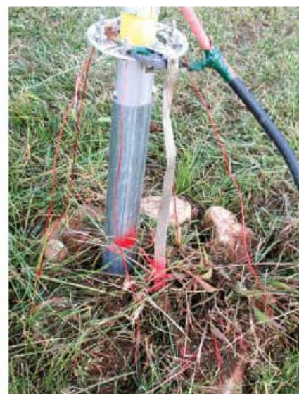
Figure 2 — The lower radial wire plate, along with the coaxial connections and ground rod cable. [Robert W. Lobenstein, WA2AXZ/9, photo]
