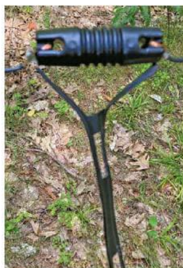
Figure 4 — Joining of wires to the ladder line.
