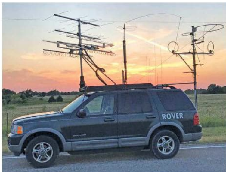
Andrea's, K2EZ/R, eight-band rover from 50 MHz to 3.4 GHz after 7 years of improvements.
