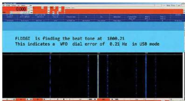
Figure 3 — In this example, the VFO is tuned to 9.999 MHz while the user is listening to WWV at 10.000 MHz in USB mode. The difference is less than 1.0 Hz, which is hardly worth correcting.
