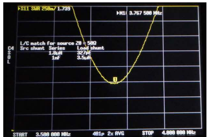
Figure 1 — The un-tuned dipole's SWR curve and L/C MATCH readings for 3.767 MHz. The middle horizontal line is the 2:1 SWR mark.
