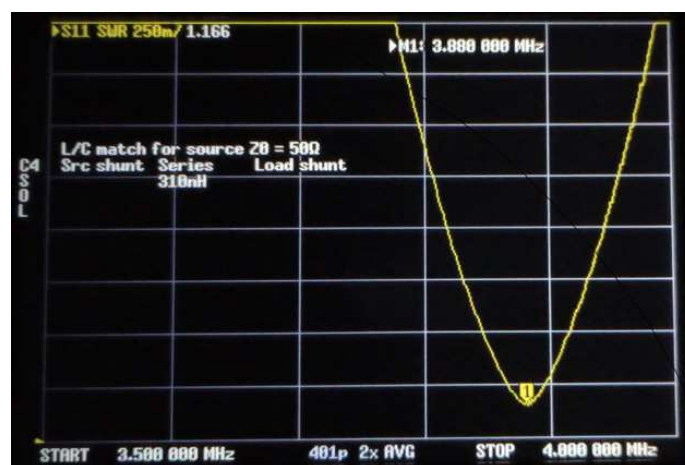
Figure 6 — The SWR chart with the antenna length shortened.
