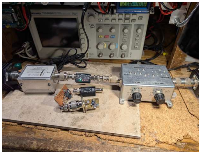
Figure 6 — The reviewer's SWR test setup.
