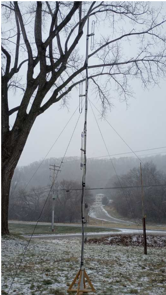
The NanoVNA's L/C MATCH function helped the author change the operating frequency of this Decibel Products DB-224.
