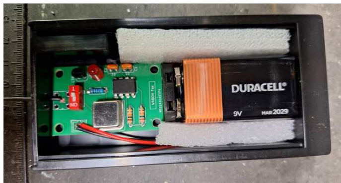
Figure 6 — The final version of the W4BOH Fox in a key-hiding container.
