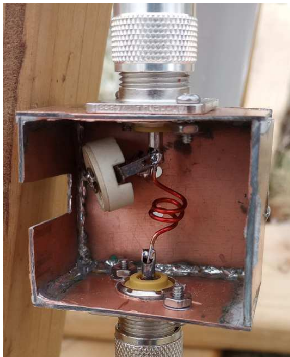
Figure 7 — The circuit constructed for the DB-224.
