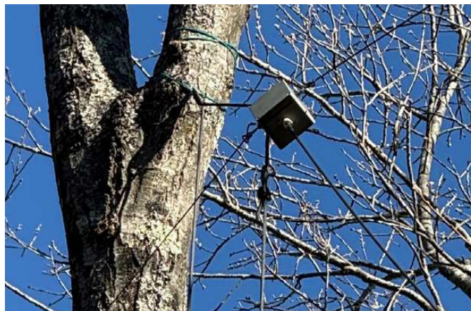
Figure 3 — The feed point of the 160-meter OCF antenna deployed 50 feet high.
