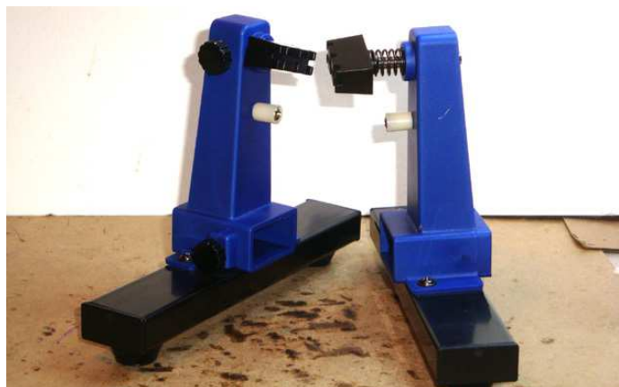
Figure 3 — The white plastic nubs shown attached to the circuit board holder's arms. [Phil Karras, KE3FL, photo]
