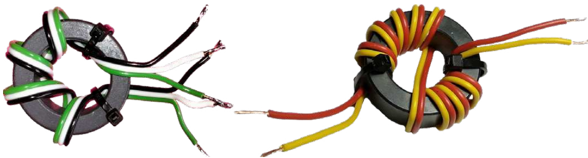
Figure 8 — Unun (T1) and current balun (T2).
