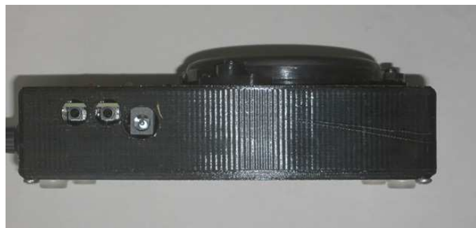
Figure 13 — Either of the two identical jacks can be used for audio in or audio out. The remaining larger jack is the power input.
