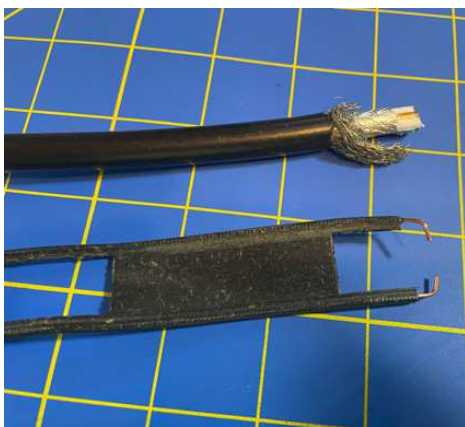
Figure 1 — Two types of transmission line: coaxial cable (top) and window line (bottom). Window line has much less loss per foot than coaxial cable, but coax is much more commonly used in ham radio due to its convenience.
