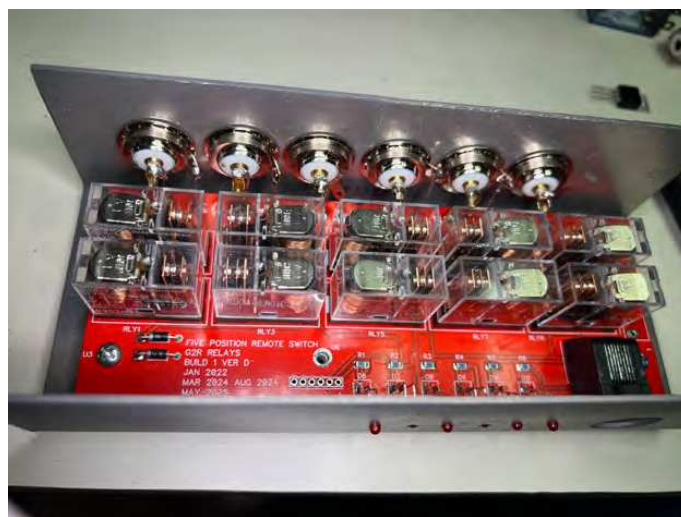
Figure 6 — Relay switch board mounted into its homebrew chassis.
