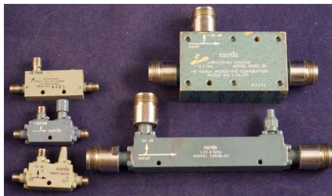
Figure 1 — Coaxial directional couplers for 10 GHz. Arrows indicate the coupling direction, and the coupling factor is marked near the top connector.
