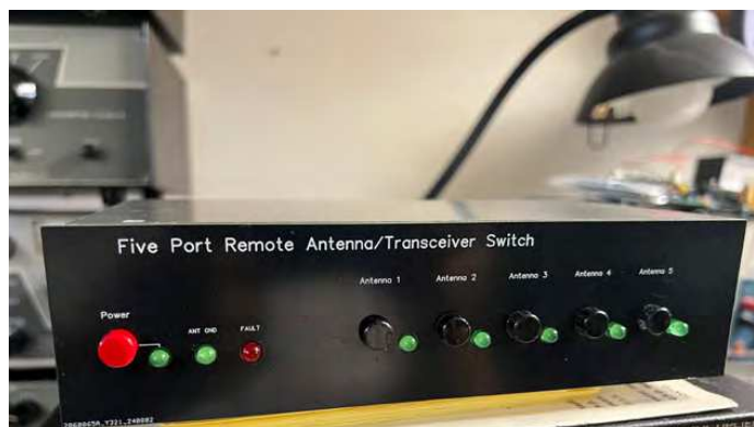
Figure 1 — The completed remote switch console.
