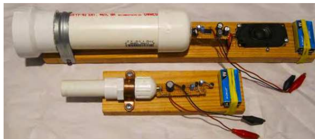
The completed transmitter and receiver, built with perforated breadboard material and wooden boards.
