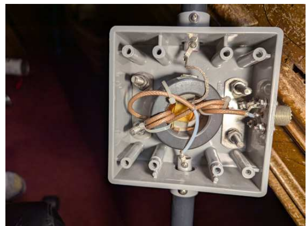
Figure 5 — The completed feed assembly for the 6-meter dipole.
