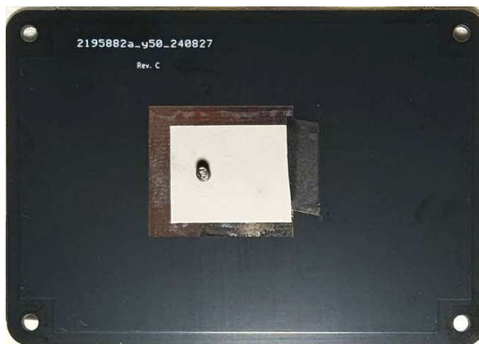
Figure 5 — Black electrical tape on the thermal pad helps to hold it in place while installing the back cover.
