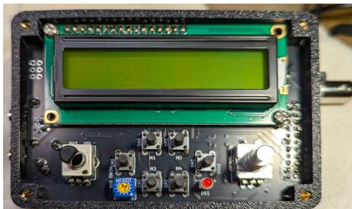
Figure 3 — The CFT1 completed display board.
