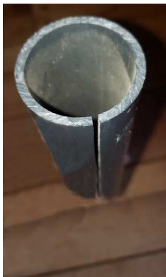
Figure 3 — The carbon fiber tube with a \frac{1}{16} -inch-long slot cut down the length of the entire tube.
