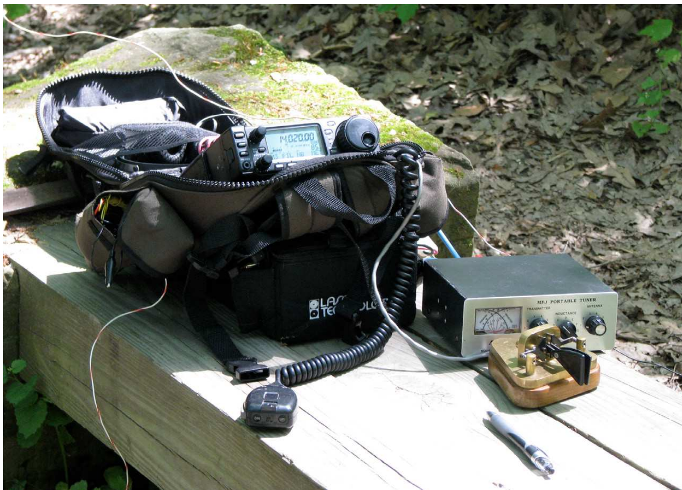
Mike's setup at the Ohio and Erie Canal: the Icom IC-703, battery, antenna coupler, and Bencher key.
