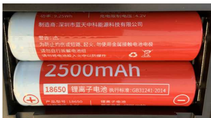
Figure 7 — The LC90 is powered by two rechargeable type 18650 lithium-polymer batteries. They may look like AAs, but they are noticeably larger.
