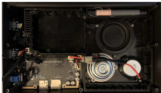
Figure 6 — The interior of the Choyong LC90. The modest ferrite-bar antenna is visible at the upper right. At the lower left is the circuit board.
