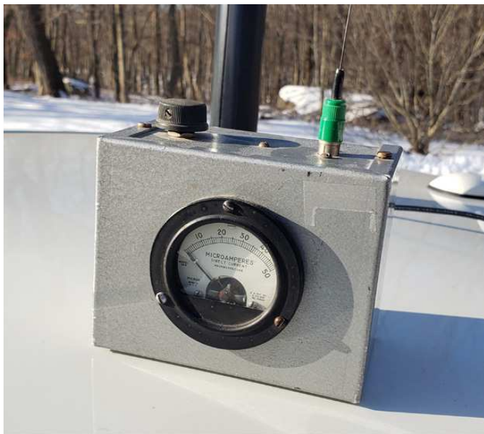
Figure 2 — The field strength meter displays no reading.
