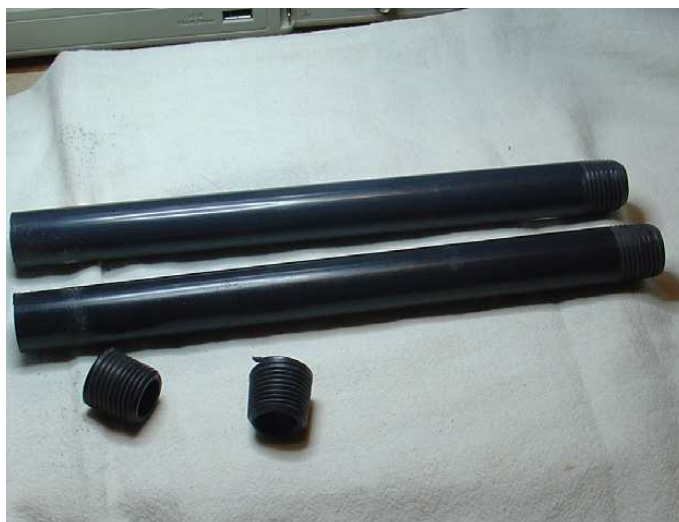
Figure 1 — PVC nipple preparation.
