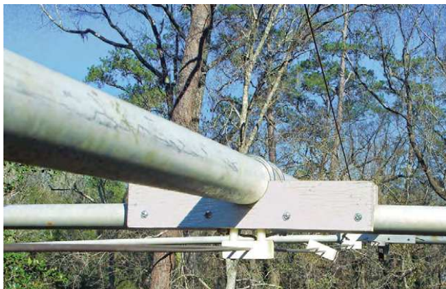
Figure 3 — The boom-to-element bracket with the feed-line spacer supported on standoffs. Just visible behind the spacer are the crossed wire jumpers from the antenna elements to the feed line.
