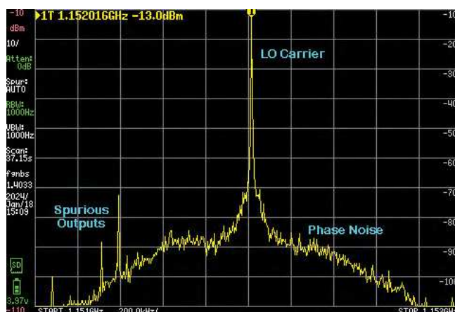
Figure 1 — Spectrum analyzer view of an inexpensive imported synthesizer signal with phase noise.
