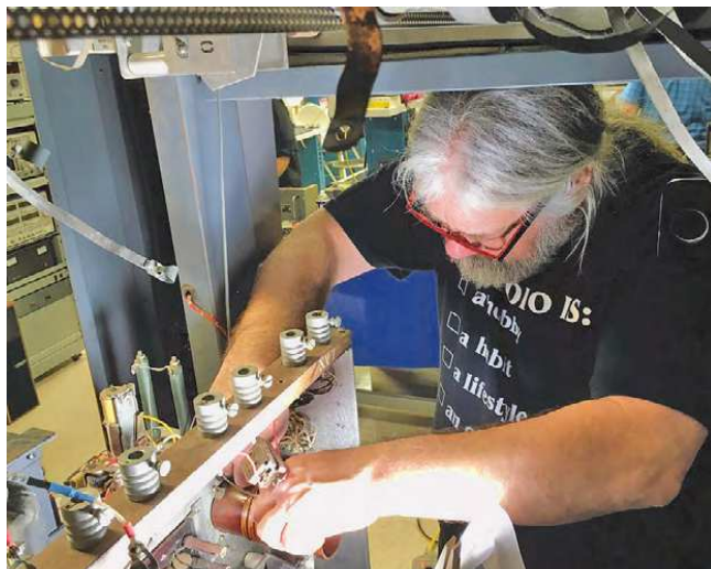
Tim “Timtron” Smith, WA1HLR, dug into the innards of the broadcast transmitter to convert it to operation on 160 and 75 meters. Click here to access an audio recording of the BC-1T’s first transmission on AM.
