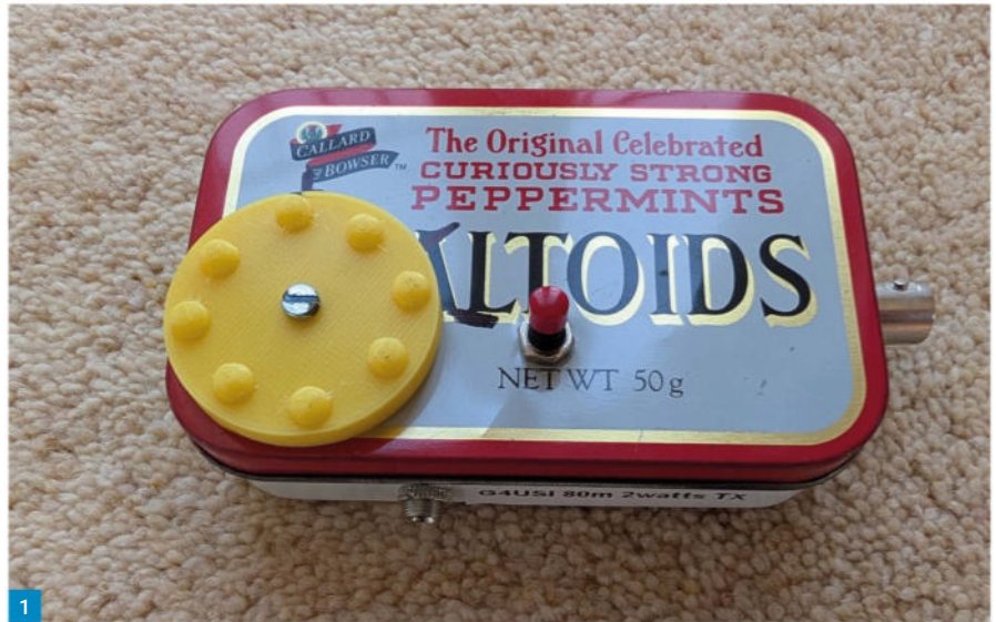
Fig. 1: The 80m CW transmitter. Tuning wheel and push switch CW key on lid. Fig. 2: 3.5mm audio socket for external key and BNC antenna socket. Fig. 3: 2.1mm coaxial power socket (or socket of your choice) and red Power LED. Fig. 4: The Kanga Mint Tin proto-board, small square side. Fig. 5: Kanga board, large square side.
