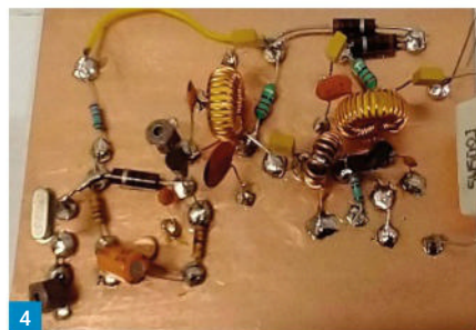
Fig. 1: A printed circuit board. Fig. 2: Matrix board or Veroboard. Fig. 3: The author's rather messy first attempt at Manhattan or Island construction. Fig. 4: A much neater version of the same project by Dave (Jake) Wills 2E0BAQ. Fig. 5: Wooden component tray. Fig. 6: The resistor colour scheme for those with 4 bands - tolerance is band 4. Fig. 7: The resistor colour scheme for those with 5 bands - tolerance is band 5. Fig. 8: The centre of a dipole. Don't forget to waterproof it!
