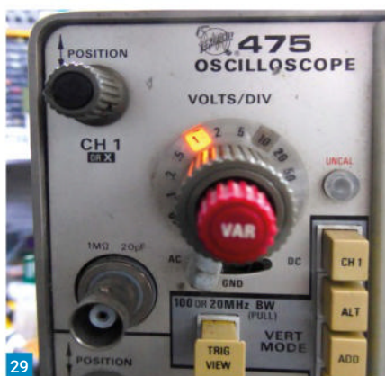
Fig. 25: Top Trigger View and Vertical Bandwidth contacts, bottom Vertical Switching 2MHz Oscillator. Fig. 26: X1 & X10 indicator bulb enclosure, Q314 & Q312 on left. Fig. 27: Grain of Wheat bulb. Fig. 28: X1 & X10 after repair. Fig. 29: X1 indicator working. Fig. 30: Dirty EHT board.
