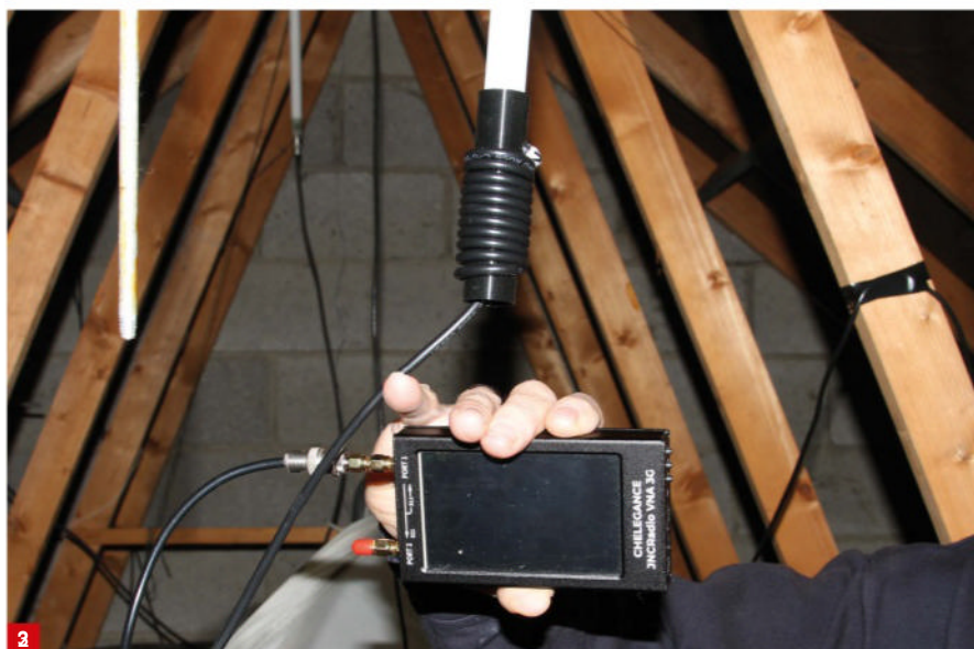
Fig. 2: VNA Measuring the Flower Pot directly at its feedpoint. Fig. 3: The Airband flower pot VNA trace at the feedpoint. Fig. 4: The antenna trace when measured at the radio end including the feeder.
