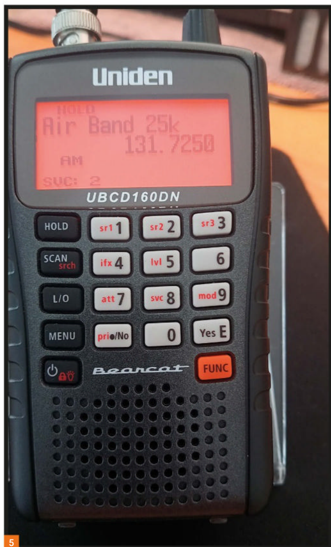
Fig. 5: The UBCD160DN was receiving one of the principal European ACARS frequencies without any problems. Fig. 6: With some auxiliary software (Zorns Lemma 11.42) the ACARS messages from the UBCD160DN could be resolved. The programme on the right of the screenshot is Friture . Fig. 7: You can use the ARC program to manage the scanner's memories and other functions.
