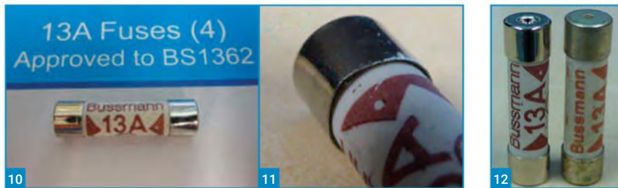
Fig. 10: Pack of supposedly conformant fuses. Fig. 11: But fuse wire trapped under cap. Fig. 12: Comparing a fake fuse with the genuine article. Figs 13 to 15: The results of testing a counterfeit fuse. Fig. 16: Incorrectly inserted plug opens access to line and neutral. Fig. 17: Similar to Fig. 16 but with a socket cover. Fig. 18: Flimsy socket cover, liable to the earth pin breaking off.
