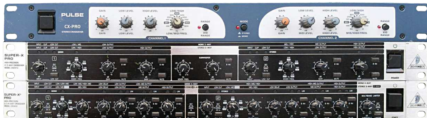
Photo 12: a selection of low-cost Chinese active crossover units. At the top is a third-order unit from Pulse; the lower black units are fourth-order LR crossovers from Behringer.
