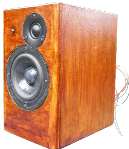
Photo 15: this speaker, based on Wavecor drivers ( PE Feb-Mar 2020) has the tweeter next to the woofer to ensure good integration up-close. No all-pass filter was necessary due to an asymmetric crossover.
