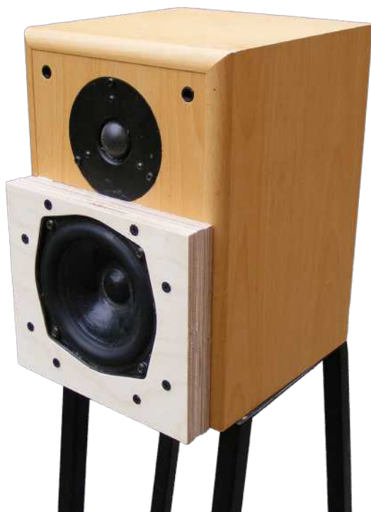
Photo 14: a stepped baffle can be used to align the acoustic radiation planes of the woofer and tweeter, but it’s a bit of a faff to build and ugly. ▼
