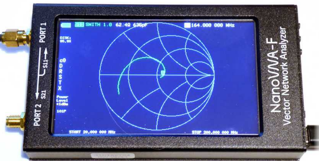
Fig.7.3: this inexpensive VNA can measure S11 and S21 from 50kHz to 1GHz.
