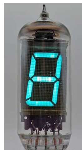
Photo 1: a vacuum fluorescent display (VFD) inside a glass tube. They also come in multi-digit rectangular assemblies. Source: https://display-tubes.org/vfd/reflector-iv-12/
