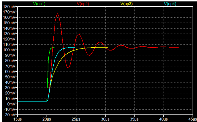
Fig.21: transient analysis (step response) for the circuits in Fig.20.
