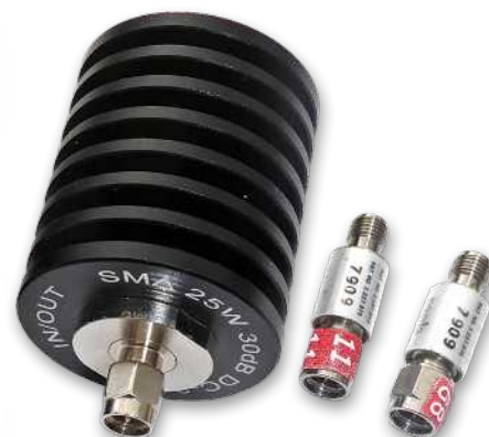
Fig.7.5: fixed external attenuators are often necessary to avoid overdriving a device and to minimise the risk of overloading the VNA's input.
