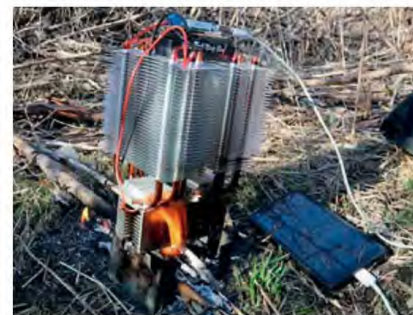
Fig.9: a DIY thermoelectric generator using an off-the-shelf Peltier device, heatsink and other components. Source: https://youtu.be/x9a2rB-xWkY
