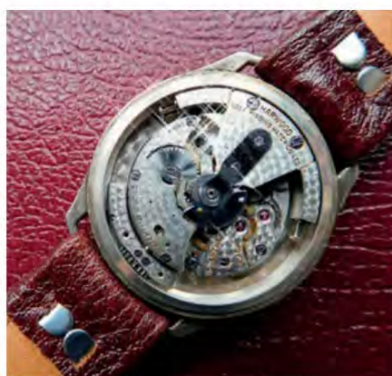
Fig.1: the first self-winding mechanical watch that harvested energy from the motion of the wearer's arm. Source: Fratello Watches – https://pemag.au/link/abxy
