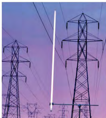
Fig.21: a fluorescent tube glowing under a high-voltage power line due to capacitive coupling of the electric field.
