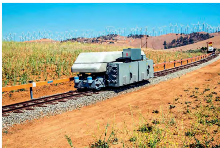
Fig.31: the ARES rail car, which climbs a hill using electricity during off-peak hours, then is released downhill during peak hours to produce energy via regenerative braking. Source: ARES North America – aresnorthamerica.com
