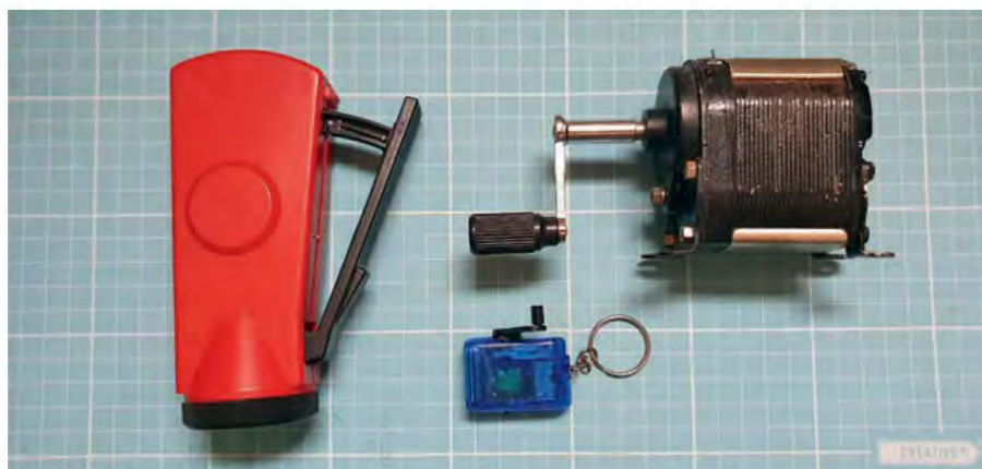
Fig.25: the Author's collection of hand-cranked devices. The red hand-cranked torch is from the former Soviet Union and has an incandescent bulb, while the blue one is a modern Chinese torch with LEDs and a reserve battery. The item at upper right is a magneto from an old telephone.
