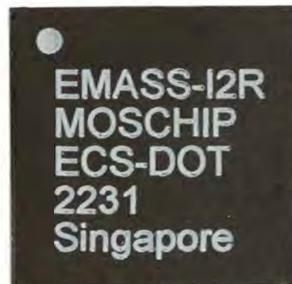
The ECS-DoT chip is shown here six times wider than in reality. It's actually only 10 × 10mm (roughly 3/8" × 3/8").
