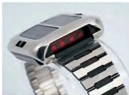
Fig.2: the Synchronar Sunwatch was the world's first solar-powered watch, released in 1972. Source: https://solarmuseum.org/cells/synchronar-2100/
