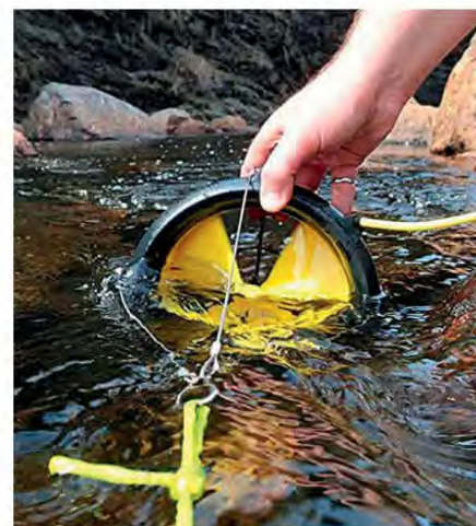
Fig.20: the "WaterLily Turbine", a portable hydroelectric generator for charging USB or 12V devices in a running stream.
