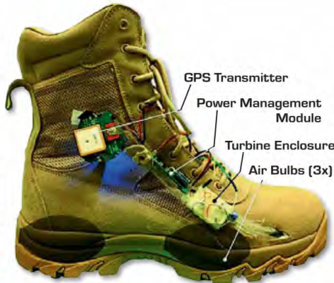
Fig.26: an energy-harvesting combat boot that powers a GPS tracker.
