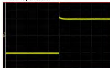
Fig.8: correct compensation is achieved when the square wave's leading edge shows no under-compensation droop or over-compensation overshoot.
