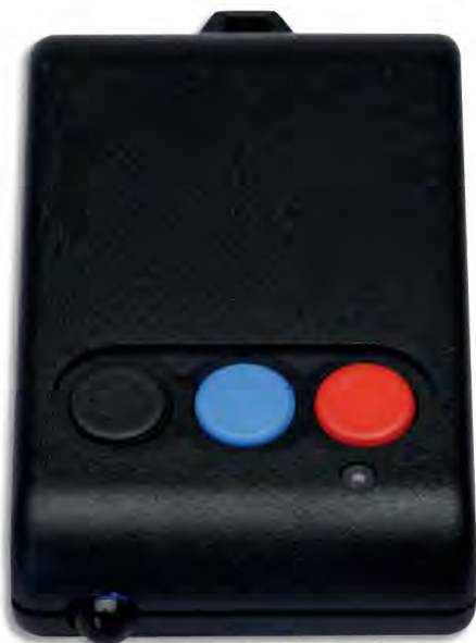
The hole shown in Fig.2 allows the IR emitter LED to poke out through the end of the case, as seen here. Note the location relative to the buttons.
