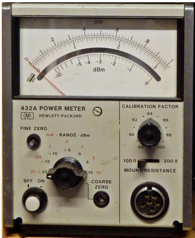
Fig.6.15: an RF power meter calibrated in RMS power and dBm.
