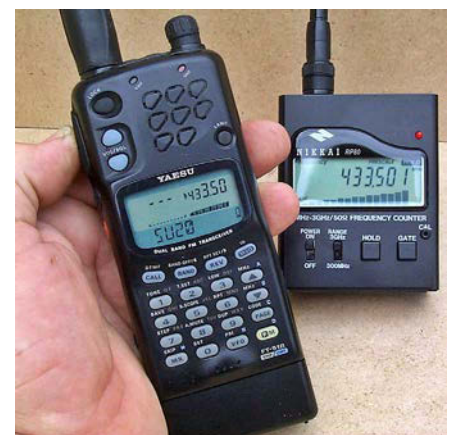
Fig.6.19: checking a dual-band FM transceiver. The DFM on the right indicates a frequency difference of 1kHz.
