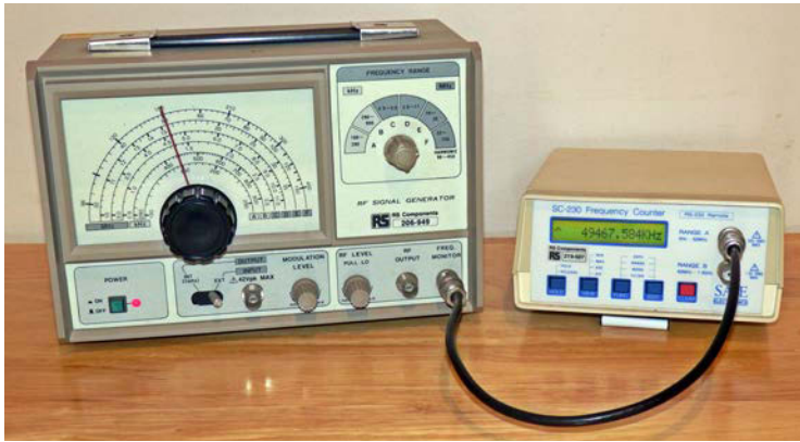
Fig.6.20: checking the calibration of an RF signal generator. The 8-digit DFM display shows 49467.584kHz with a 1Hz resolution.
