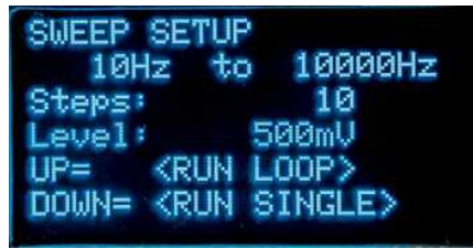
Screen 11: SWEEP uses the UP, DOWN and OK buttons like the OUTPUT mode. There is the option of running a single sweep pass or performing a continuous loop.
