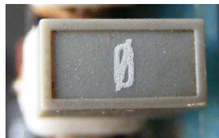
Photo 1: the polarity inversion button on a mixer channel strip.
