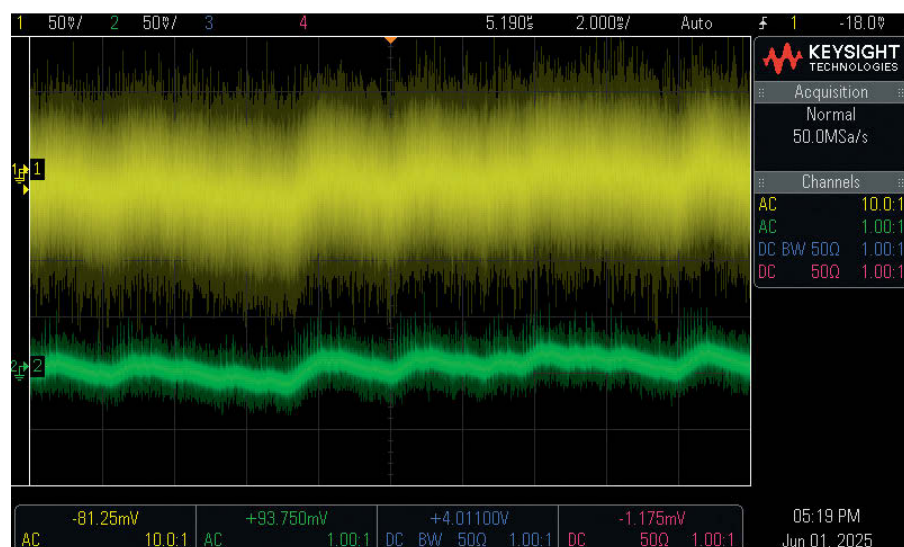
Scope 1: the results from the test shown at upper left. The waveform measured by the standard probe (yellow trace) is completely buried in switching noise, while the green waveform from the Power Rail Probe is much more informative.
