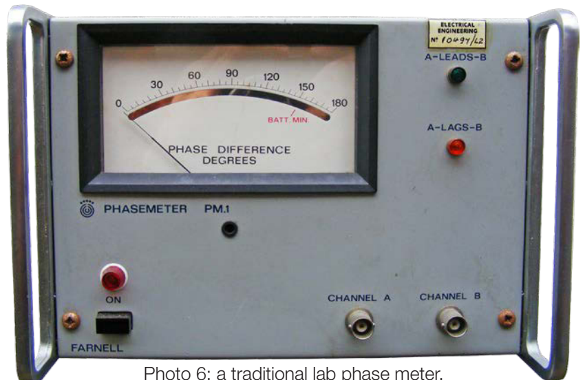
Photo 6: a traditional lab phase meter.
