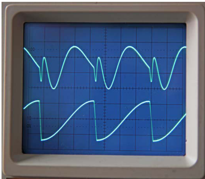
Photo 7: the result of phase-shifting a wonky ramp.
