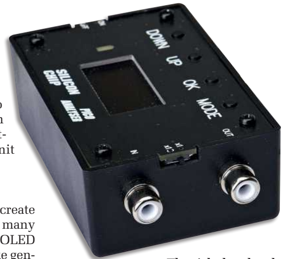
The right-hand end of the case has two holes for the RCA sockets and a notch for S6.
